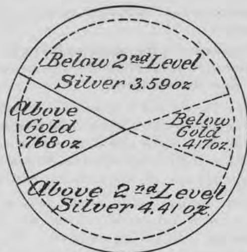
Fig. 5. Diagram showing variation in vertical distribution of gold and silver in Lone Pine mine. The solid lines apply to values, above No. 2 level, and the dotted lines to values below No. 2 level. Wedges show relation of gold to silver in each. Diagram based on average values in ounces per ton.
